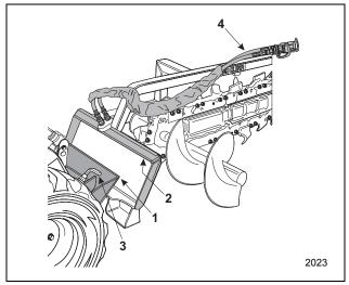
Figure 3–26 Hydraulically Powered Attachment Installation
